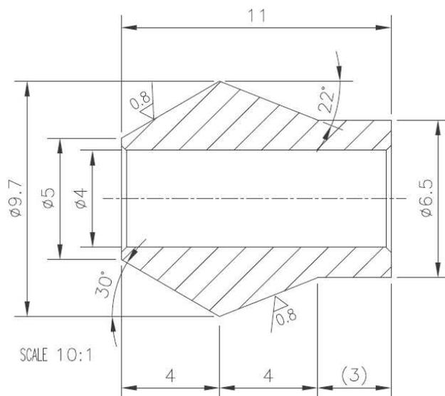
You need to use the cone in the picture above on a hole of about  $\varnothing 6 - \varnothing 7$  with sharp edge, place on the same axis of the transducers hole, i.e. of the fillet
